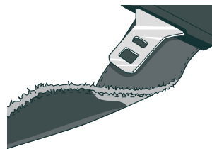
FIGURE 5: Example of a fraying seatbelt
